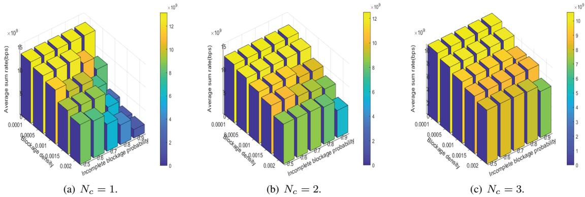
Fig. 3. Impact of blockage density and incomplete blockage probability threshold on average sum rate.
