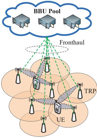
Fig. 1. Architecture of coordinated multi-beam transmission in mmWave networks.
