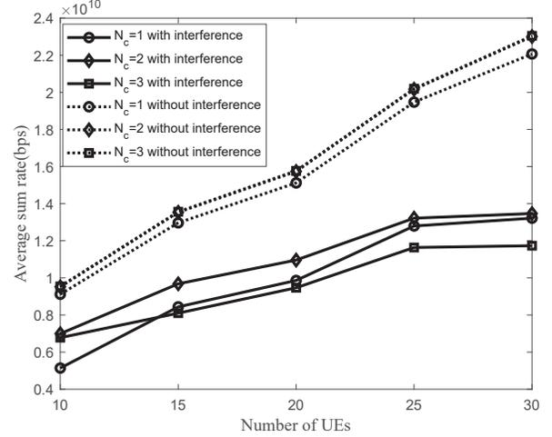
Fig. 2. Impact of different numbers of coordinated beams of each UE on average sum rate.
