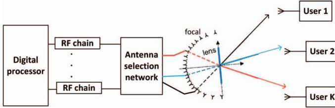
Fig. 1: Diagram structure of mmWave MU-MIMO with lens antenna array at BS.
