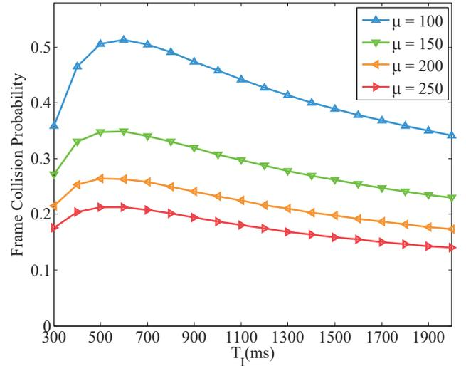
Fig. 5. Frame Collision Probability Versus  $\mu$  and  $T_I$
