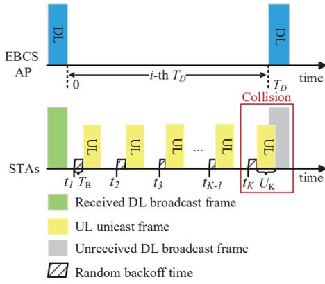
Fig. 3. Frame Collision between DL Broadcast Data Frame and UL Unicast Data Frame Within  $T_D$
