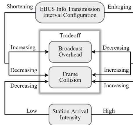
Fig. 1. Tradeoff Among EBCS Info Frame Transmission Interval, STA Arrival Intensity, and Frame Collision
