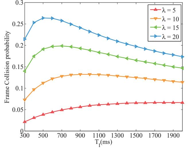
Fig. 4. Frame Collision Probability Versus  $\lambda$  and  $T_I$
