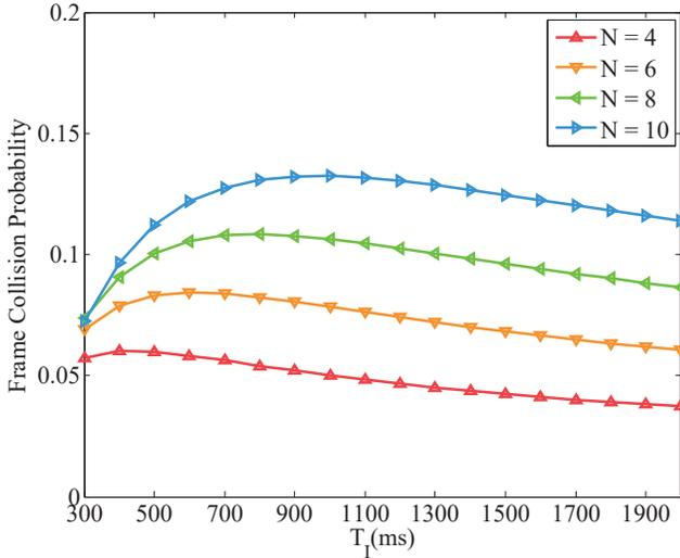
Fig. 6. Frame Collision Probability Versus  $N$  and  $T_I$
