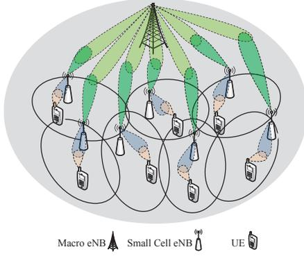
Fig. 1. UDNs with wireless mmWave self-backhauling.
