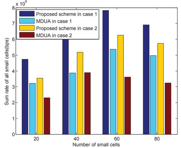
Fig. 3. Sum rate under the proposed scheme and minimum-distance based user association with different numbers of small cells.
