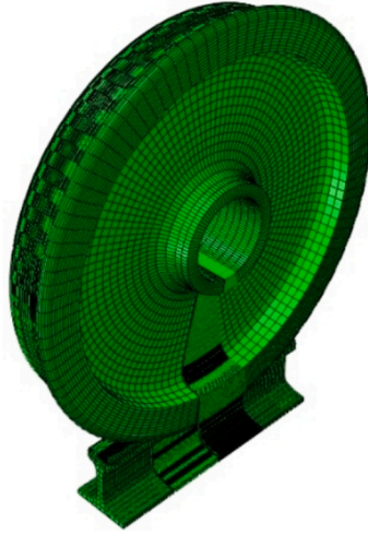
Fig. 8. Finite element model of wheel-rail contact.
